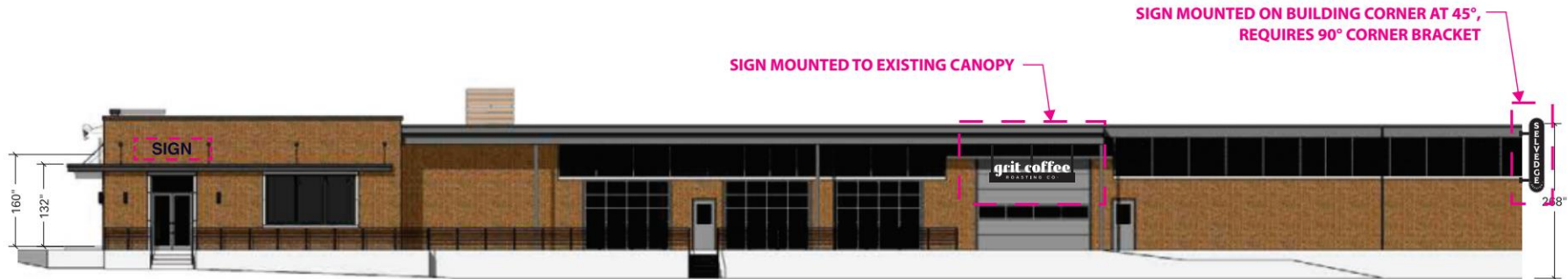
2 EAST ELEVATION - BUILDING SIGN AREA
